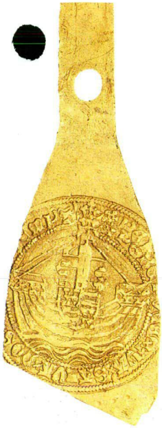
Above. The gold trial plate of 1477, the earliest in existence. Trial plates provided the means whereby the accuracy of the gold coinage could be checked against an officially-approved standard.
