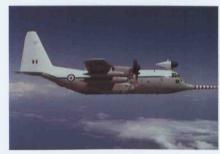
The Meteorological Research Flight uses a Hercules aircraft to carry out research into the effects of clouds on atmospheric radiation from the sun and infra-red radiation from the earth; the physical characteristics of cloud formation at all levels; and the chemistry of the lower part of the atmosphere.
