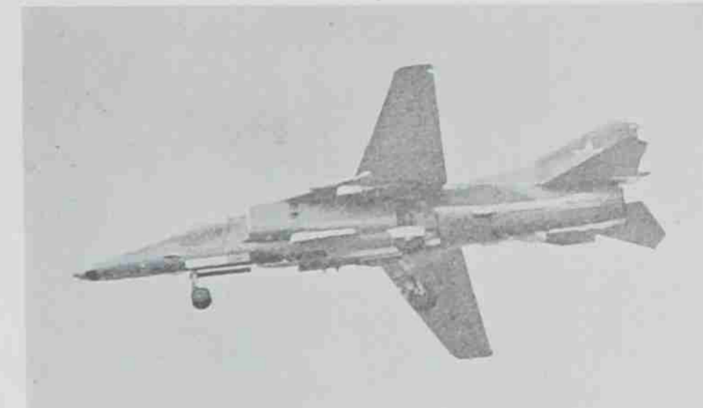
▲ Soviet Flogger D swing-wing specialised ground-attack aircraft
