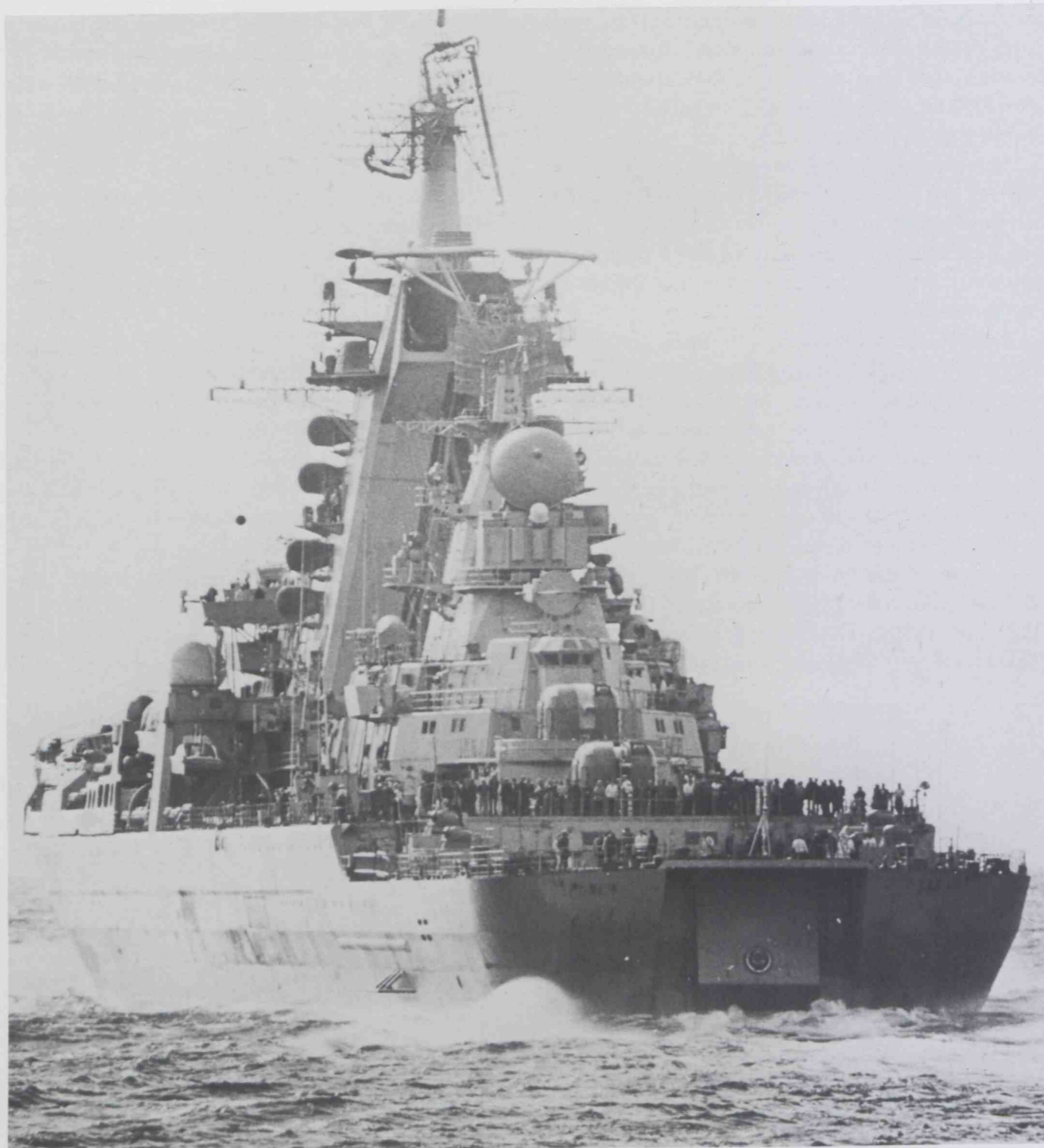
In this view from astern, the nuclear-powered guided missile cruiser KIROV reveals a superstructure massed with radars and electronic sensors, a stern door for ASW sonar, helicopter deck bordered by Gatling guns and 100mm dual purpose gun mounts.
