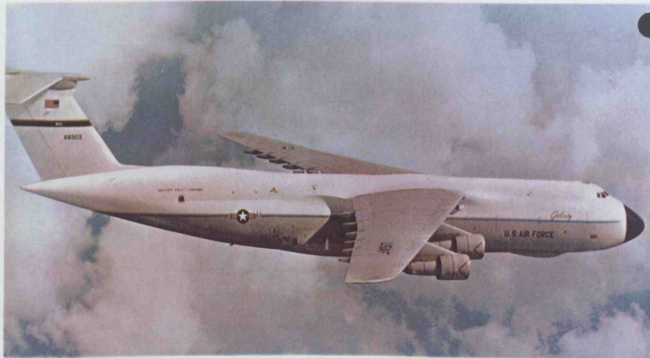
C-5A GALAXY MILITARY TRANSPORT PLANE—the main aircraft for rapid movement of heavy arms to theaters overseas. Range, with full load of 100 tons, is over 6,000 km.
