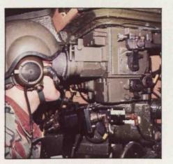
Installation is completed by placement of an armoured 'D' piece in front of the sight, positioning of the armoured cowl, and attachment of the electrical connection and ballistic link
