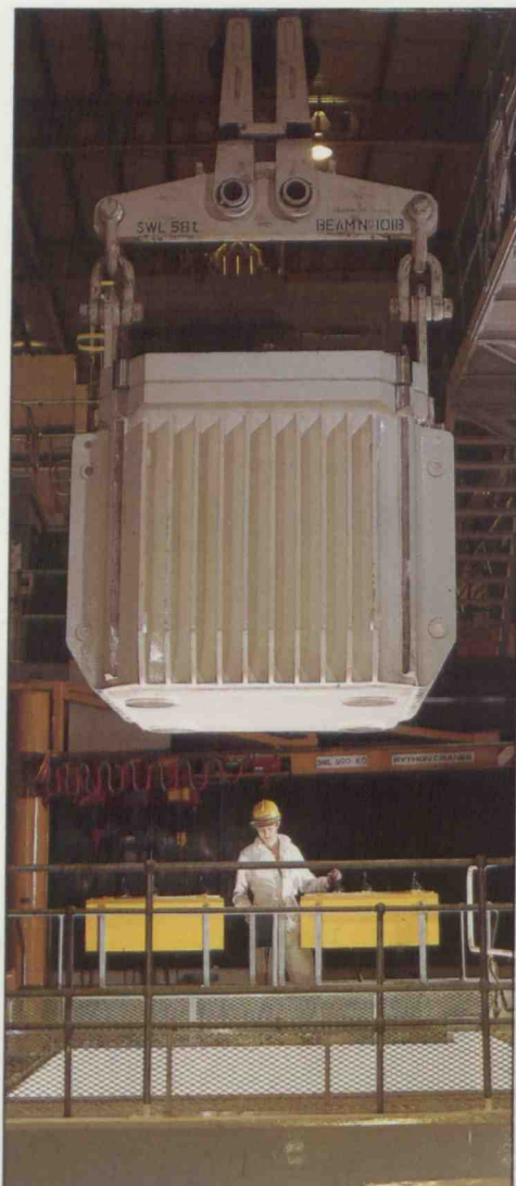
Flask being lowered into an inlet cell.
