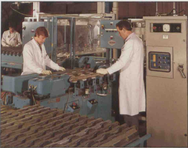
Welding the ends of Magnox fuel elements.
